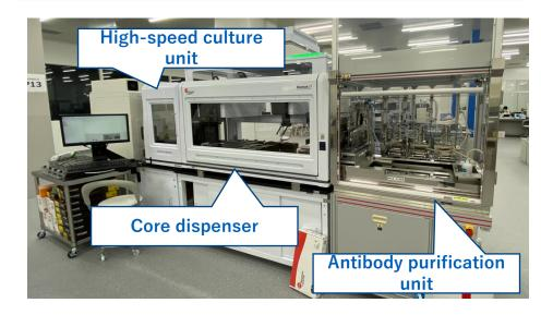
Cell culture (left) and antibody purification (right) experiments are done by one dispenser (middle). This has increased utilization and investment efficiency.
